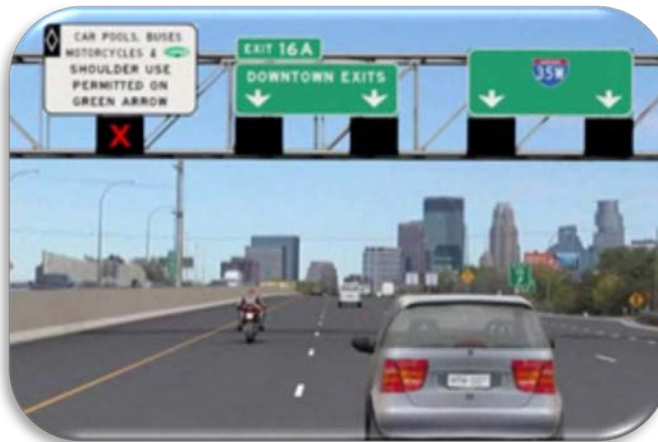
Figure 14. Graphic. Closed Priced Dynamic Shoulder Lane—Minneapolis, Minnesota. (27)
